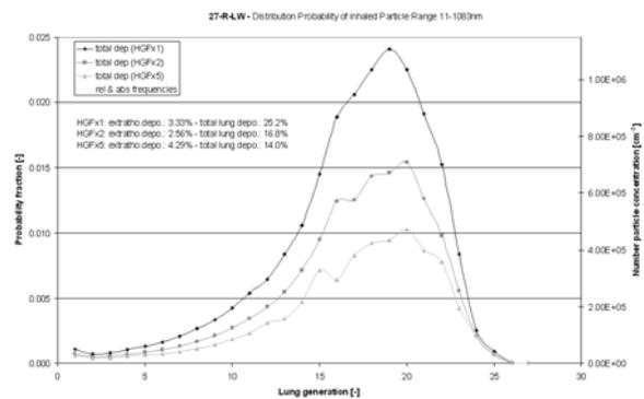
Figure 2. Modelled deposition pattern of the end-of-stack aerosol, using the Monte Carlo code IDEAL. Plotted are three individual simulations for various Hygroscopic Growth Factors (HGF).
