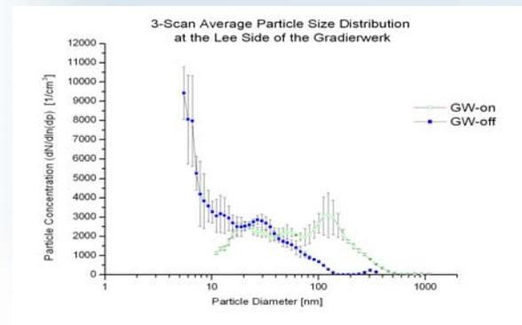
Fig. 3: Differences in particle size distributions during on/off cycles at the lee side of the GW, representing a 3-scan average with standard deviation
