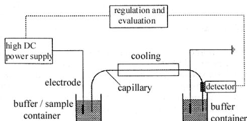
Fig 1.1 Capillary electrophoresis (CE) system for the analysis of anions
