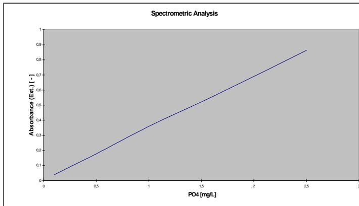
Fig 2.1 Chart of photo-spectrometric absorbance of phosphate with increasing concentrations (dilution series) (see also appendix-tables for a more detailed chart)
