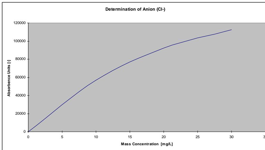
Fig. 1.5 Chart of Chloride absorbance versus mass concentration (for a more detailed display, see appendix)
