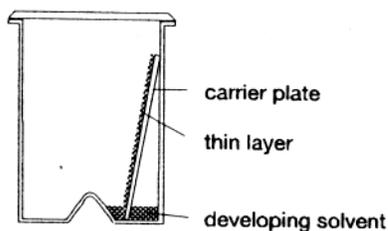
Fig 3.2 Development chamber for TLC
