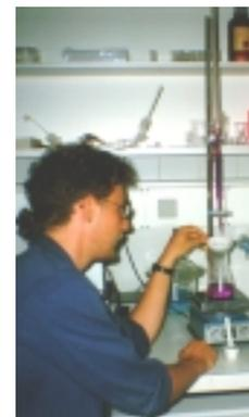
Fig 4.1 Titration and boiling procedure with KMnO<sub>4</sub>
