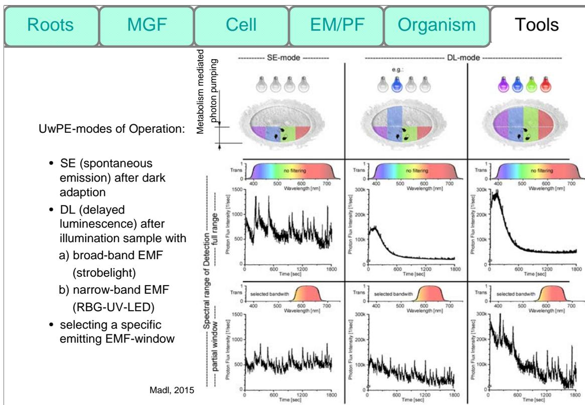
Upon placing a biological specimen into the detector chamber, as conceptualized in Figure 2, two modes of operations are possible. The first concerns activation of the sample with a light source (delayed luminescence, DL-mode) prior to measurement, whereas the second operates without an external light source and aims to detect spontaneous emissions (SE-mode).
