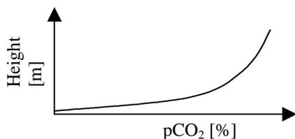
Height of tower versus CO<sub>2</sub> concentration; the optimum is achieved in towers that do not exceed 20m in total height.
