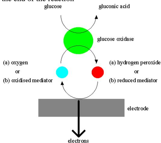
↑ Glucose Oxidase Sensor (GOD). glucose reacts with the oxidised form of the enzyme to form gluconic acid, but leaves behind two electrons and two protons, thus reducing GOD. Next, oxygen dissolved in the surrounding fluid reacts with GOD, accepting the aforementioned electrons and protons to form H<sub>2</sub>O<sub>2</sub> (hydrogen peroxide) and regenerating oxidised GOD- which is ready to react once more with glucose.
