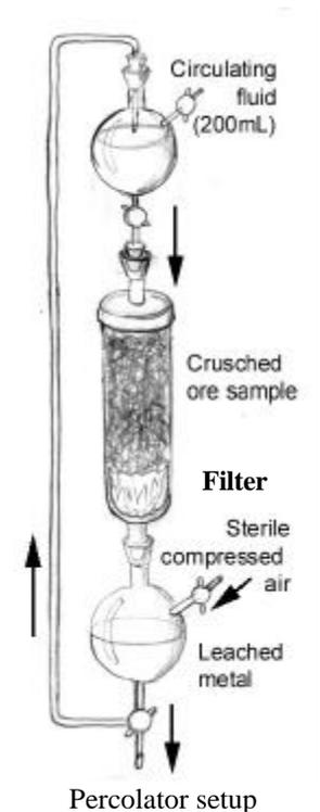
**Bioreactor:** mining industry design bioreactors, where  $O_2$ ,  $CO_2$ , and pH can be accurately set; “**Air Lift Reactor**”: Supply of microorganisms with needed air occurs simultaneously and the suspension of finely grounded substrates; i.e. mud waste. Up to 2 tons per load can be processed. Current models are capable of handling up to 200 tons per leaching event.
