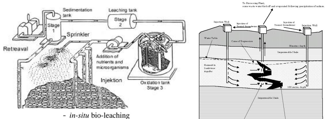
Generalized cross section of *in-situ* leaching process applied to a sandstone hosted roll front type uranium deposit (South Australia) ®
