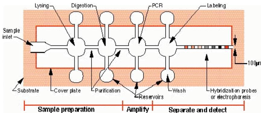
→ Conceptual design of DNA processing and analysis chip.
