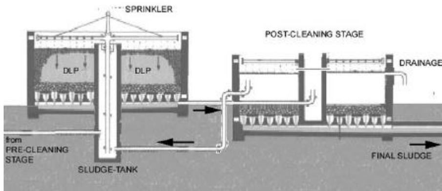
Technical realization of DLP: The wastewater is sprayed onto the trickling filter bed; the organic matter adsorb to the grid and microbial growth takes place.
