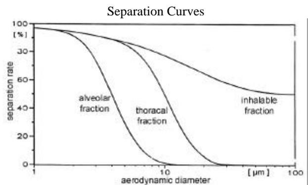
Fig.3: The separate fractions for the inhalable, thoracic and alveolar portions of airborne dust within the respiratory tract; because of the logarithmic representation an aerodynamic diameter " zero " is not representable; for which a separation rate of 100%.
