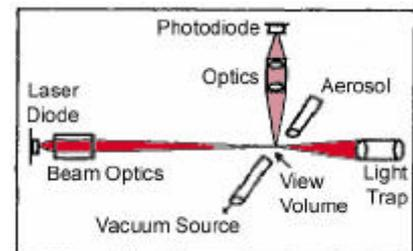
Fig.4: Basic design of an OPC
