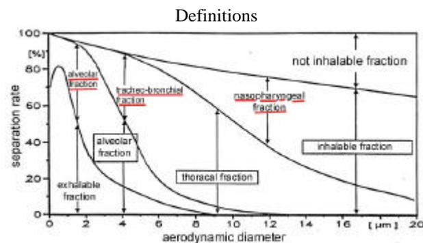
Fig.2: Aerosol fractions as a function of the aerodynamic diameter; medically relevant deposited aerosol fractions according to the industrial standards are underlined; the framed proportions relevant for the measuring techniques contain also their respective exhalable portions.
